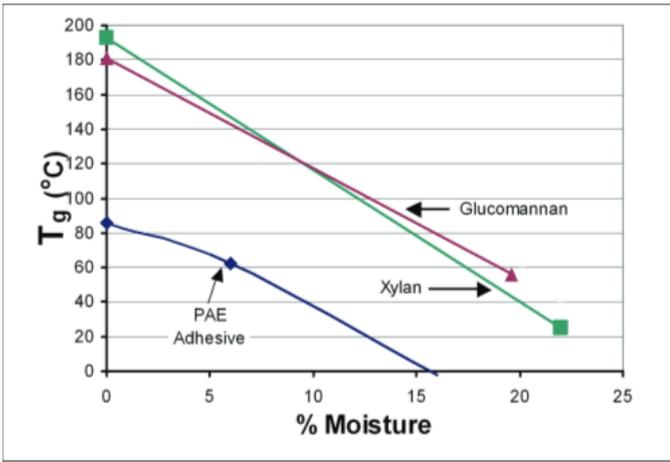
Figure 8 – Impact of moisture on coating  $T_g$  (Furman 1993)
