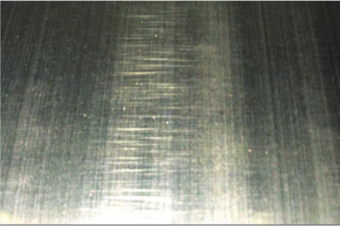
Figure 3a - Band of dryer surface chatter
