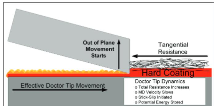
Figure 6a - High resistance to MD movement encountered
