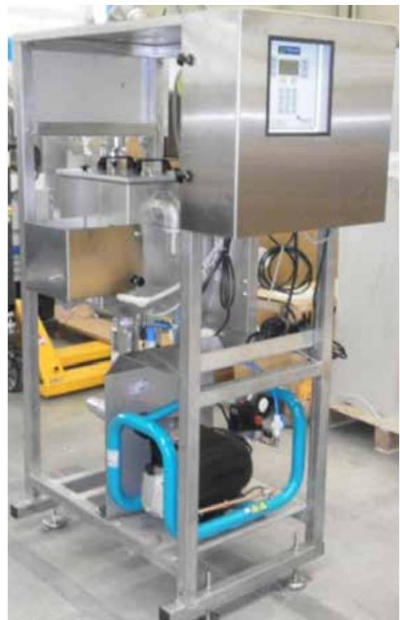
Figure 1: 3D TRASAR Caster Technology Unit
